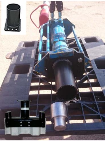
The Atlas Copco PD1 is not only a very compact units, but the combination of it and its very portable hydraulic powerpack provides a substantial advantage over conventional air powered equipment.
