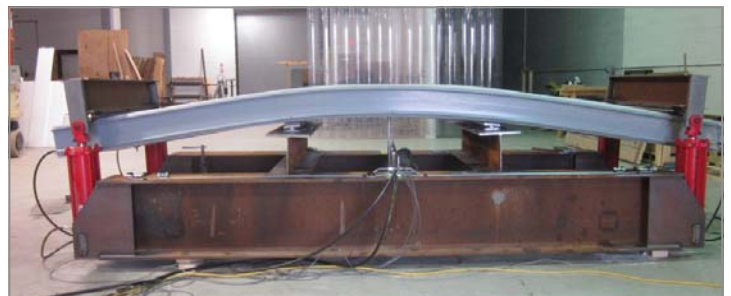
8" thick specimen at full cylinder travel
