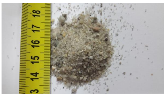
Photo C.1 The masonry sand
