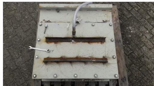
Photo 3.4 Test box closed with detachable lid
